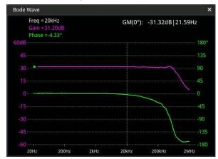
The purple line in the picture is the frequency graph, straight as a ruler from DC to >200kHz.
